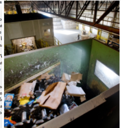
Sorting machinery is seen in operation at ecomaine, which is the company Waterville contracts with to dispose of its recyclables. The company says it will no longer accept plastic retail and grocery bags because the items clog up the sorting machines at its recycling facility in Portland. Contributed photo by Brian Fitzgerald
